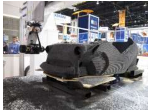
Strati – phase 2 subtractive manufacturing
